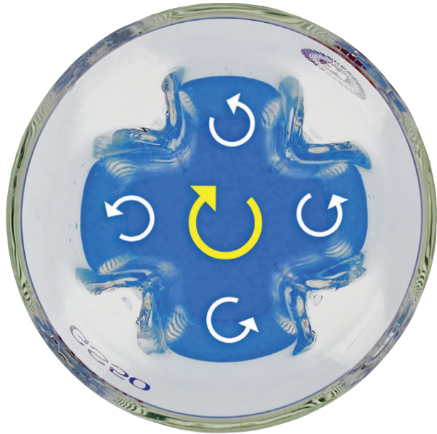
GS vessel principle (viewed from top)
